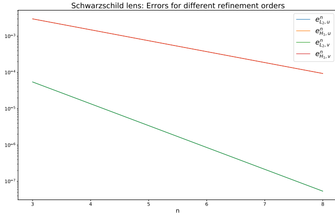
Fig. 3. Schwarzschild lens error: L_2 and H_1 errors for different refinement orders with Dirichlet boundary conditions. The orange and red lines overlap, as well as the green and blue line.
