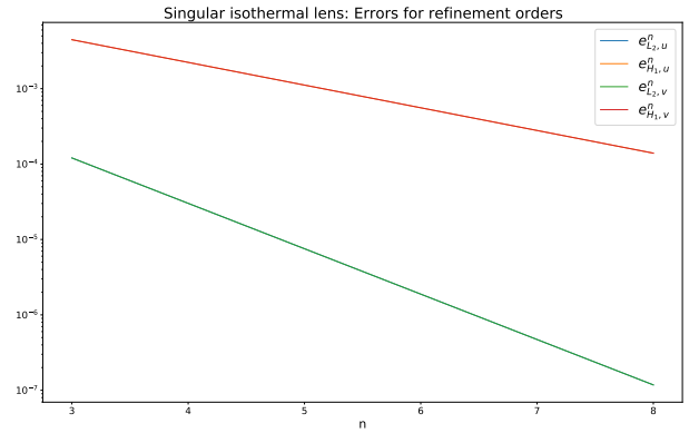
Fig. 5. Singular isothermal lens error: L_2 and H_1 errors for different refinement orders with Dirichlet boundary conditions. The orange and red lines overlap, as well as the green and blue line.
